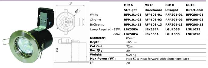
Available in a variety of attractive finishes this high quality straight or directional downlight is ideal where the lighting requirement should be fire and acoustic rated. Its shallow design depth of 100mm allows for installation into very small ceiling voids and is suitable for domestic, commercial, retail and many other building types.
